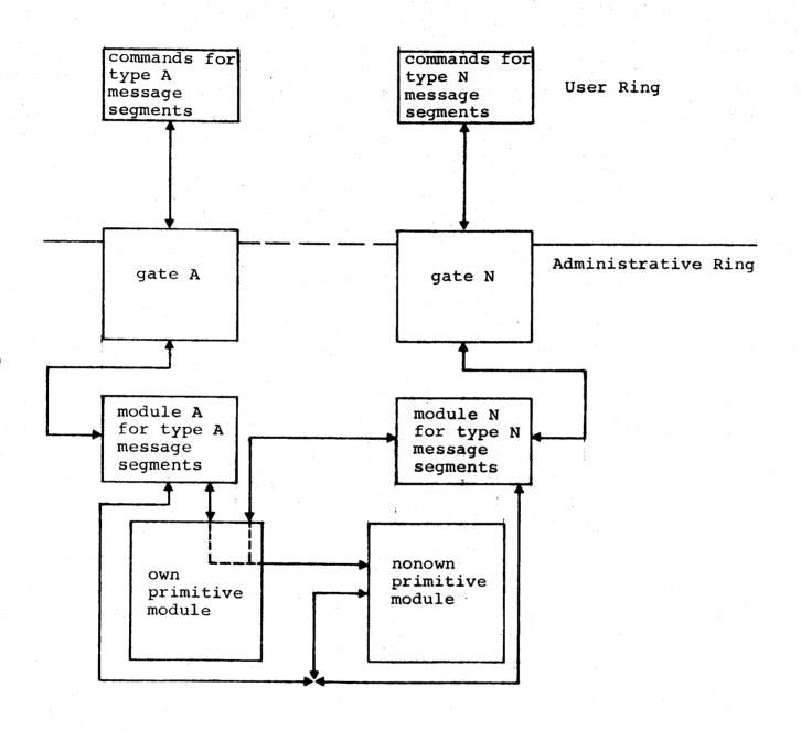
Figure 2-1. Sample Message Segment Facility Configuration
